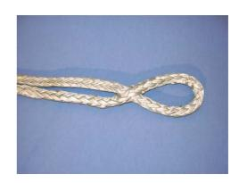
4. The end is buired in the middle of rope. 10 braids is recommended length
