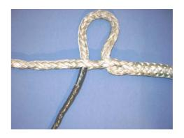
7. The rope's end is tapered down to a very thin end. Tapering should be about 20-30 times the diameter of the rope
