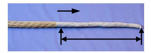
8. To finish the splice the end is threaded into the center of the rope. Begin to thread 4 braidings from the last stitch
