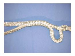
2. Open the rope where the eye starts and mark the size of the eye
